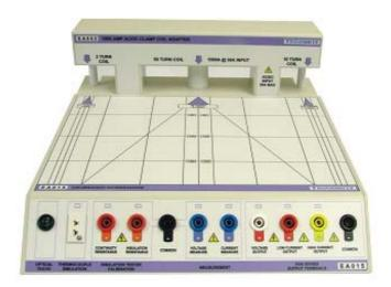
The multi function workstation provides a central work area with all connections routed conveniently to remote terminals mounted at the front of the adapter.
