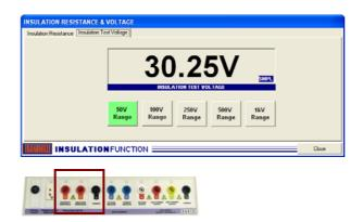
Connect meter to terminals marked Insulation resistance.
