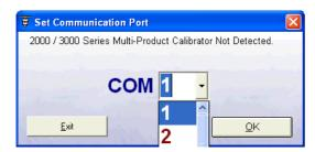
On starting the virtual front panel for the first time, a COM port selection screen will be displayed. Click on the COM port that is connected to your 3000 Series calibrator to continue.
